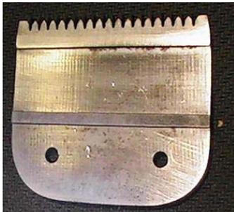
The cutting surface of the Andis 8 1/2 blade has very short comb teeth. This style does not let the many types of coat enter the blade very well. In my experience, Cockers, Chows, Cats, Schouzers, some Poodles, the blade seems to drag somewhat and pushing the clippers makes it more difficult.
