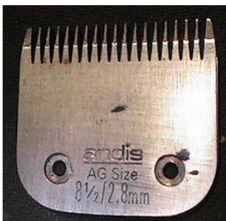
The back of the Andis 8 1/5 blade has seemingly long comb teeth, but they are not recessed enough to the cutting surface to cut difficult coat. See picture above again, short stubby teeth.
