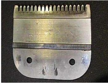
The cutting surface of the Oster 8 1/5 blade has longer teeth letting more hair into the comb for cutting. On this particular blade it will be easier to push through most types of coat because of the depth of the comb teeth.
