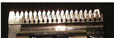
When the cutter is placed back on the Andis 8 1/2 blade correctly, only the tips of the cutter do any cutting. Hair can bunch up at the front of the blade because the cutter isn't cutting it fast enough with just the tips of the cutter, so the blade drags in some coats. The cutter should slice the hair not rip at it. When the blade heats up that cutter may move because of metal expansion. If it goes forward it may cut skin, if it backs up it will stop cutting altogether.
